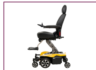
Drives Safely at 4mph While Elevated at 12"
