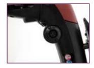
Dual Charging Ports Can Charge Battery Pack On/Off-board.
