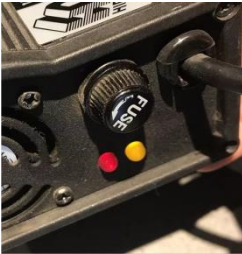
Yellow light: Charging
