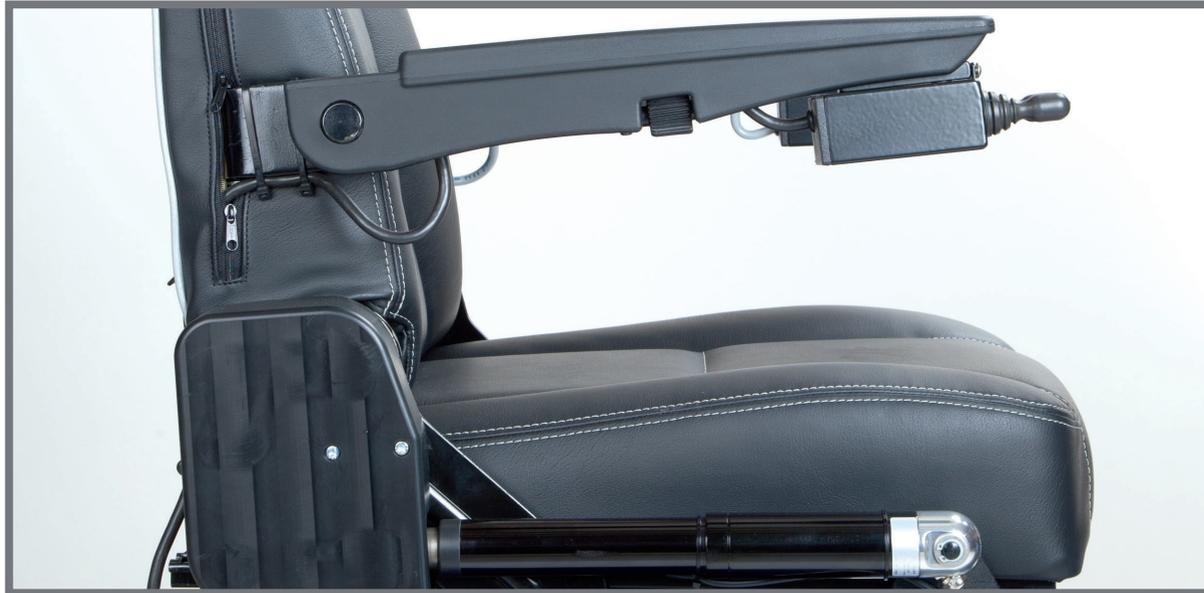
Electric seat tilt - max weight 27.7 st (175 kg)
