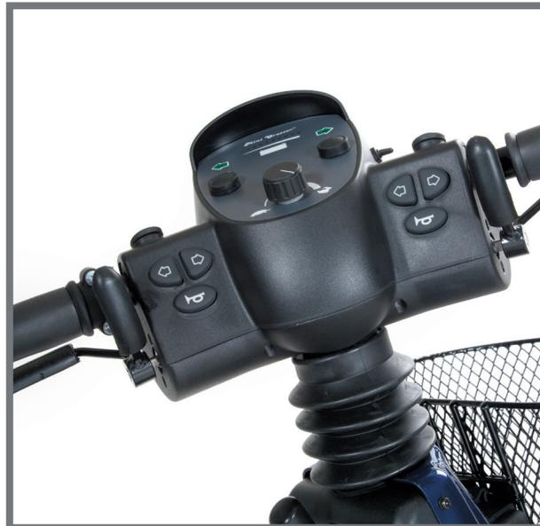
Left and right accelerator, with switch
