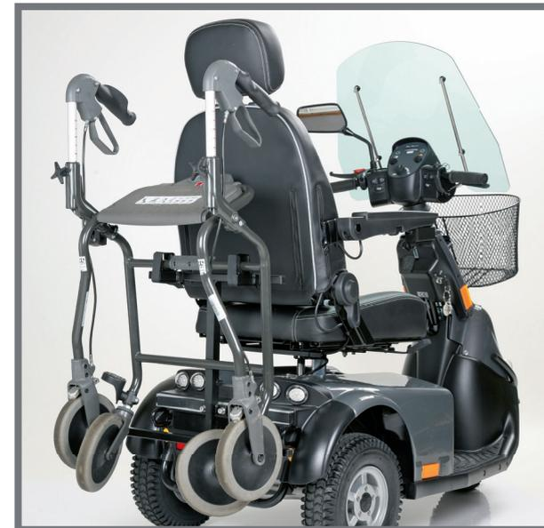
Rollator carrier, Max weight 20 kg
