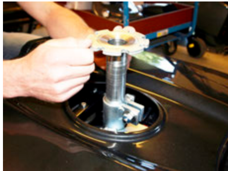
Adjust the seat post height to the desired position. The seat post is marked with a ring for each centimetre.
