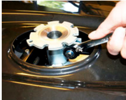
Unscrew the contra screw. Use the combination spanner, 17 mm.
