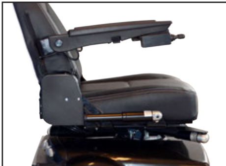
Seat in outer back position. (Can be adjusted 15 cm)
