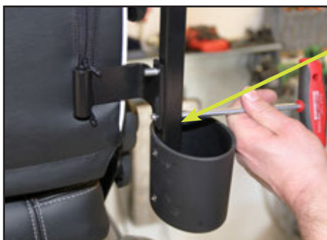
Secure the walking cane holder using two screws. 6 mm head.
