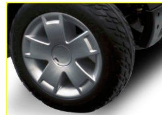
10" Alloy Style Pneumatic or solid Tyres (solid tyres only available in black)
