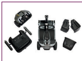
Easily Disassembled Into Five Pieces
