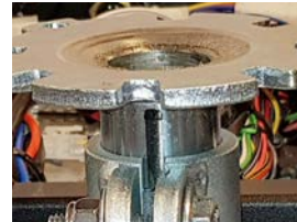
Be aware that the black line is holding its position after movement, so the seat is straight in front of the steering.
